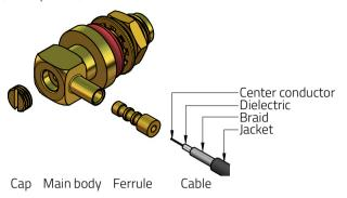
**Step 2.** Pre-tinned cable conductor (optional), make sure no evidence of melting Slide ferrule onto cable until cable jacket reach internal positioning point
